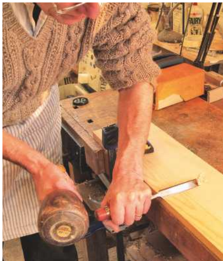
▲ Pic.3 Taking an angled cut down to the line
